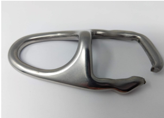
Highly ductile failure of an austenitic 316L stainless steel piece
