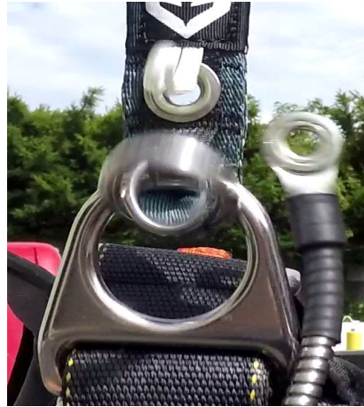
3-Ring Assembly at time of cutaway release
